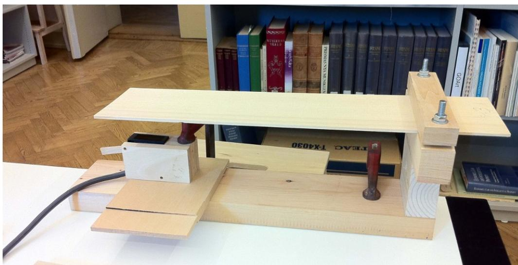
Sample clamped in the fixture with the laser displacement recording its rest position before starting tests.
