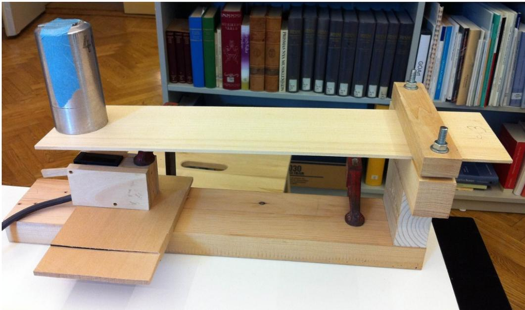
Measuring the sample's bending at the given position.
