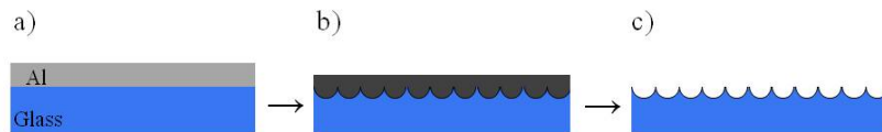
Figure 3.13: AIT process scheme: a) as-deposited Al on glass, b) same sample after annealing and c) resultant glass after etching.
