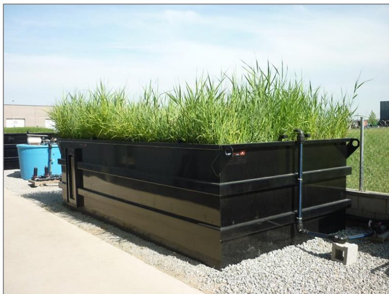
Figure 5.3. View of the VFCW pilot
