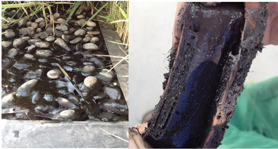
Figure 5.22. Deposit accumulation in the inlet (HFCW) and in the dripper emitters (IP)
