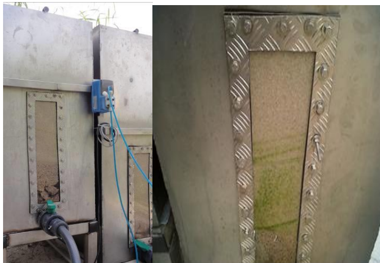
Figure 3.7. VFCWs media layers
