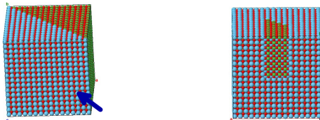
FIG. 4: Super-cell with a displacement (1/2, 1/2, 1/2) in direction [0\ 1\ 1] . FIG. 5: Super-cell with a displacement (1/2, 1/2, 1/2) in a small region.
