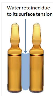
Fig. 12. Water surface tension between ampoules
