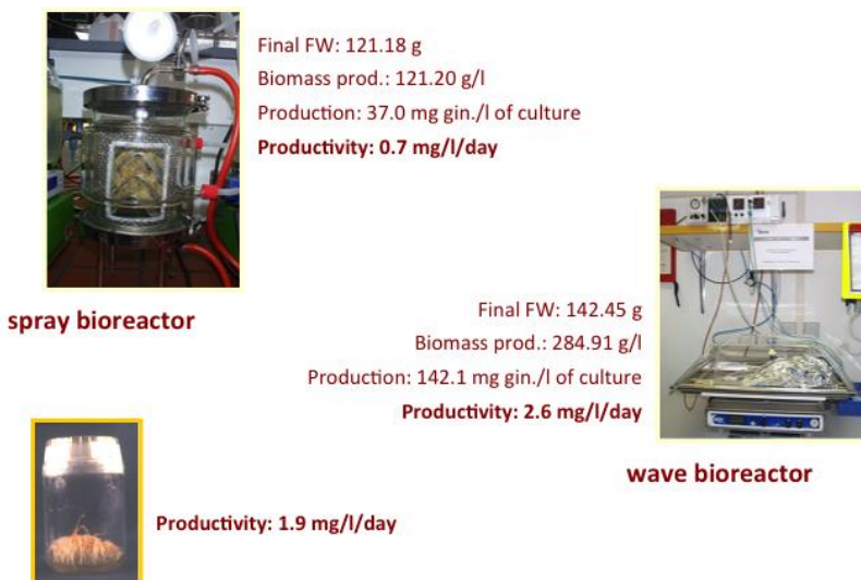
Figure 13. Ginsenoside productivity of typical hairy roots (HR-M) grown in small flasks, spray and wave bioreactors on a 56-day culture with change of media every 15 days.
