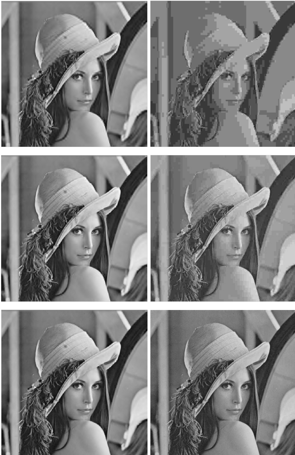
Figure 5.2: Lenna's image compressed using JPEG 2000 (left) and JPEG (right) at rates 0.0625 (up), 0.125 (middle), and 0.25 (down).
