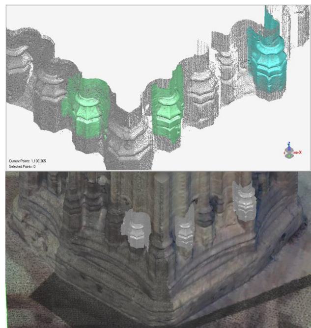
Figure 2. OS mesh placed on TLS point cloud (Cathedral of Seville)
