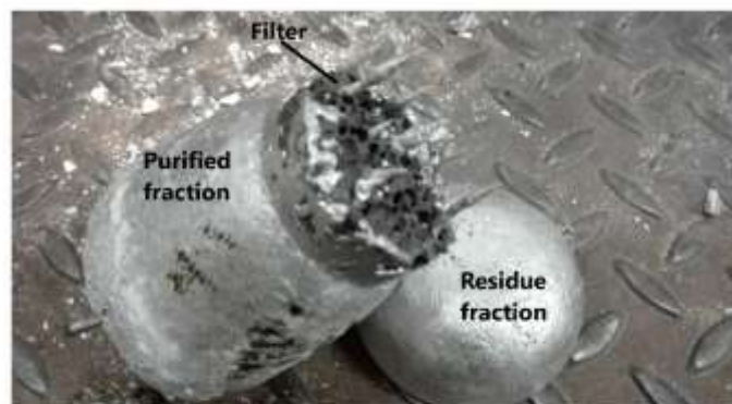
Figure 21. photo of an example of the purified fraction that solidified on top of the filter, and the enriched liquid fraction (residue) that passes through the filter and solidified in the reservoir.
