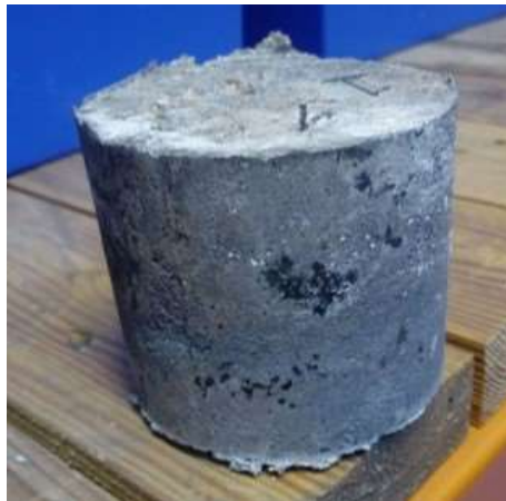
Figure 24. Cylindrical purified sample, cut from the filter, obtained at the end of the process.
