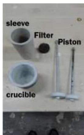
Figure 18: Filtration experiment components: a crucible is used to melt the alloy. A sleeve is inserted in the crucible and a filter is placed inside the sleeve. The piston is used to squeeze the semisolid alloy to the filter through the sleeve.
