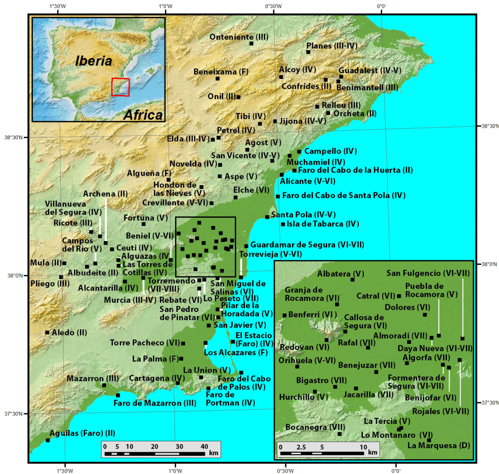
Figure 2. Macroseismic intensity map for the main events. As these events occurred just 18 minutes apart, it is impossible to disentangle their macroseismic effects and the map should be look as the joint result of both. Intensities are evaluated in EMS98.
