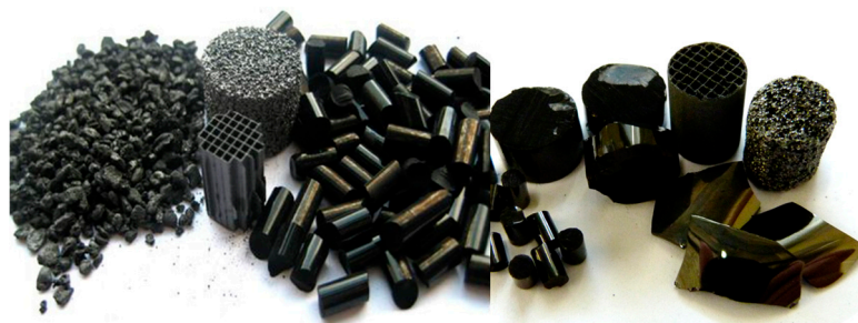
Figure 1. Carbon materials obtained in different formats: grains, powders, pellets, films and coatings on monolith and foam structures.
