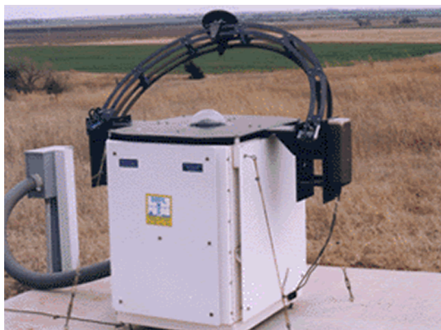
Fig. 2. Day/Night WSI fielded at SGP CART site.
