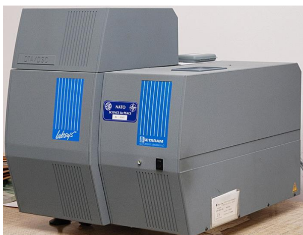
Figure 3-30. Instrument utilized during DTA/TG analysis, Setaram Labsys DTA TG (DEMaC, University of Aveiro).
