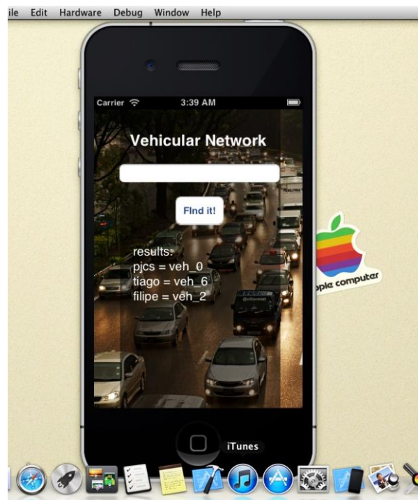
Figure 23 - VNS consumer app for iOS: this screen shows the emulator running the consumer application for VNS. Below the button we see a list of associations user-vehicle, returned from the server. This list contains the most recent ID of all the OBUs each user connected to.
