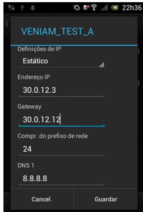
Figure 15 - OBU/Rabbit Address - Dynamic mode: If the OBU address field is left empty, the system will use the gateway's address by default. The image on the right shows a manual configuration of the network, however it equally works using DHCP
