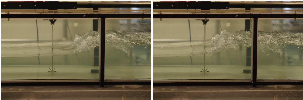
Figure 4. Positive surge propagation above the large roughness element - Flow conditions: Q = 0.061 \text{ m}^3/\text{s} , d_1 = 0.155 \text{ m} at x = 5.9 \text{ m} , Fr_1 = 1.39 , Tainter gate opening after closure: h = 25 \text{ mm} - From left to right: 0.121 s between successive photographs (shutter speed: 1/400 s)
