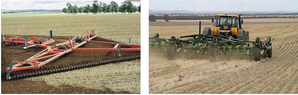
Figure 32 (Left) - a Brookfield disc cultivator used for full cut tillage. (Right) – A disc planter designed to plant with minimal soil disturbance and full stubble retention (photos from manufacture’s website)
