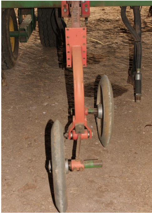
‘Figure 3 Press wheel located behind knife point (photo courtesy of Neville Gould from Conservation Agriculture and No-till Farmers Association, Wellington NSW)
