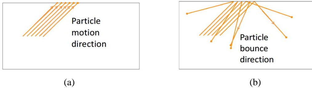
Figure 4.9. Two boundary conditions. In the figure, dots denote particles and solid lines denote particles' trajectories. (a) Stick boundary, (b) Diffuse- reflection boundary.
