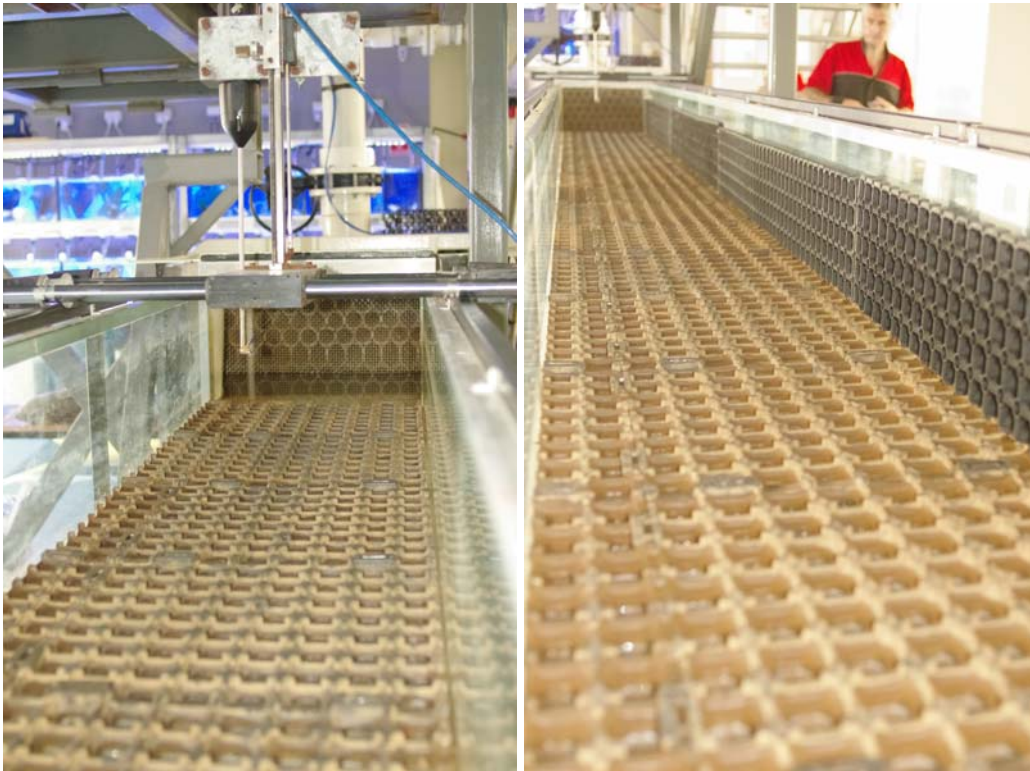
(A) 12 m long flume looking upstream; (Left) Rough bed configuration - note in the background the intake structure, the upstream screen and flow straighteners behind; (Right) Rough bed and rough left sidewall configuration
