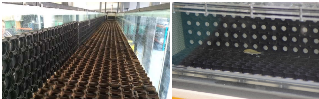
(C) Configuration 3: rough bed, and combination of rough and smooth sidewall
