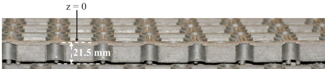
(C) Rubber mat used in the water tunnel and along the 12 m long flume sidewall
