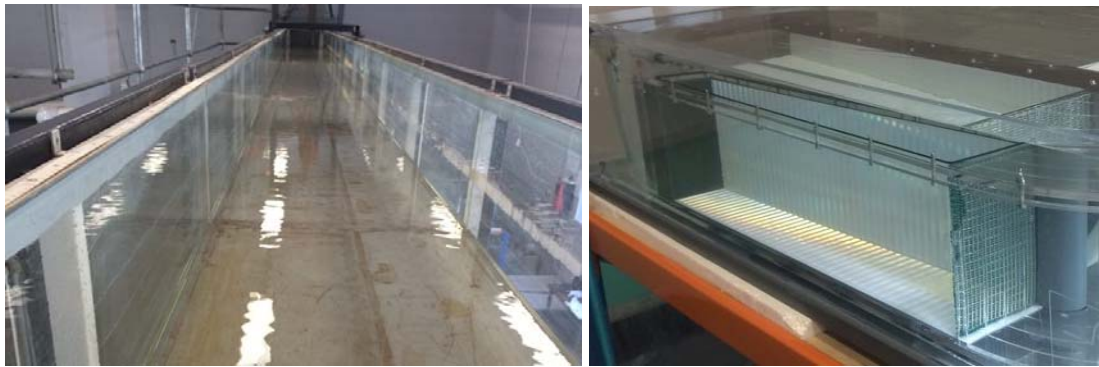
(A) Configuration 1: smooth bed and sidewalls
