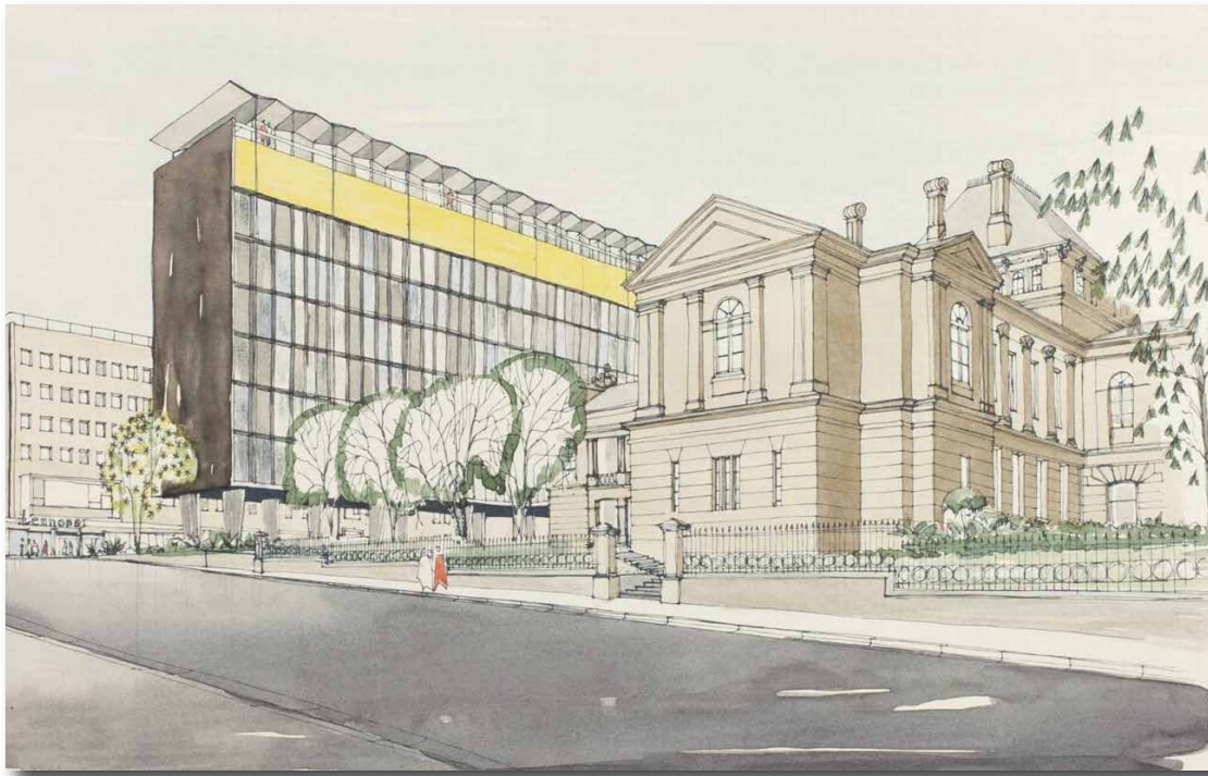
Above: Perspective view from Ann Street and North Quay of FDG Stanley's Supreme Court building for which a design remained undocumented. With no prospect of promotion at the Commonwealth, Pavlyshyn was co-opted and rapidly designed a modern, multi-storey slab block, elevated on pilotis along the George Street alignment with underground parking. This would satisfy the functional shortfall and leave untouched the exterior of Stanley's Courts while providing access to its garden, now uncluttered with cars. The interior was sympathetically reworked.
