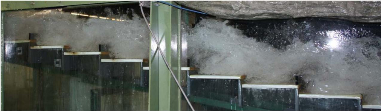
Fig. 3. Air-water flow patterns on stepped spillways with embankment dam slopes
