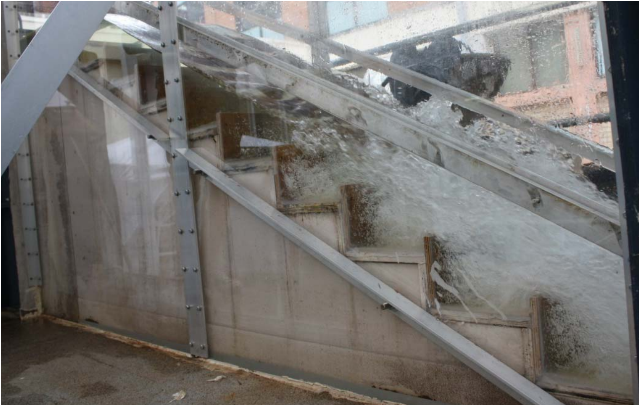
Fig. 3. Air-water flow patterns on stepped spillways with embankment dam slopes
