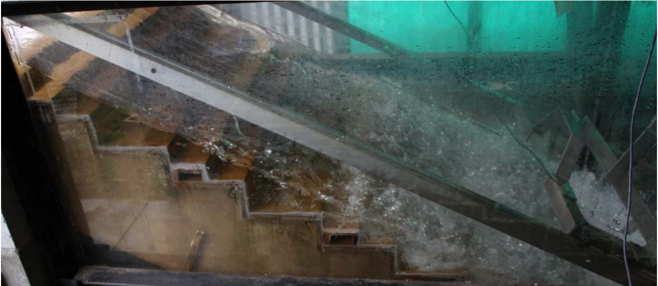
Fig. 3. Air-water flow patterns on stepped spillways with embankment dam slopes
