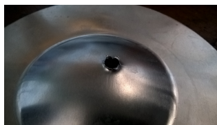
Figure 12. The influence of the piercer on the diaphragm.
