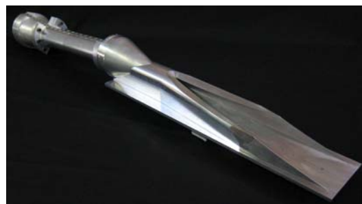
Figure 3 M12REST engine half-scale model. From [6].
