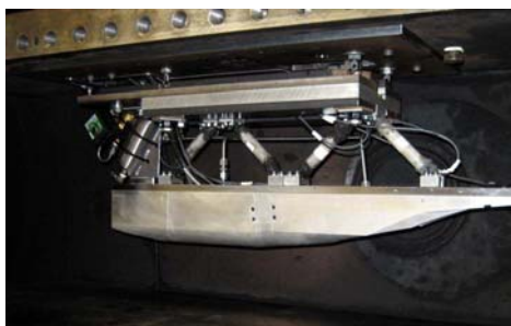
Figure 2 M12REST engine 0.32 scale, attached to multi-component force balance. From [14].
