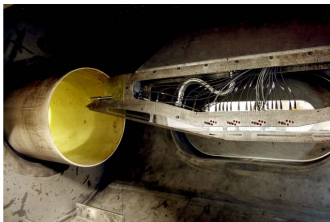
Figure 5 Mach 10 2-D Scramjet inside the X3 expansion tube. Side covers are removed showing the internal instrumentation.
