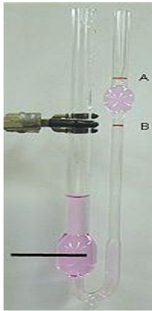
Figure 2 Ostwald viscometers measure the viscosity of a fluid with a known density (268)
