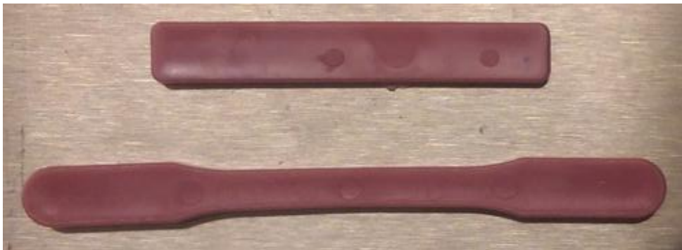
Figure 1. Rectangular section and tensile test samples for composite batch 2
