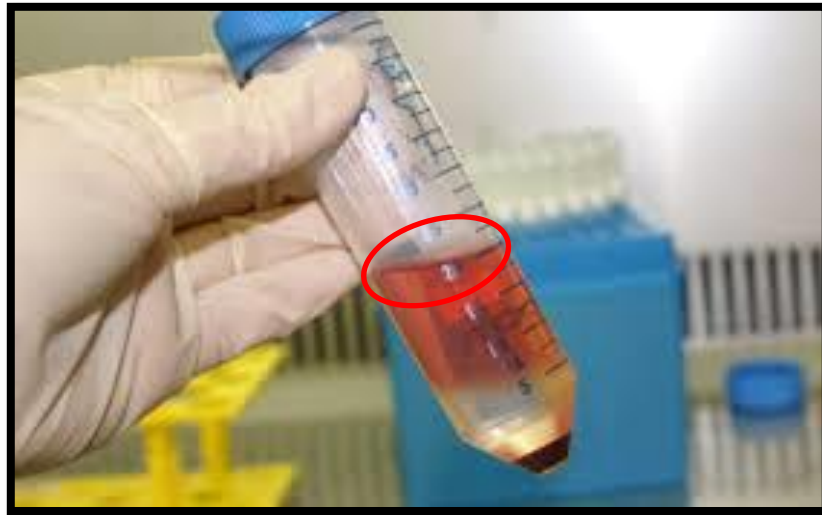
Figure 9.3: The PBMC interface layer between the plasma and Ficoll after centrifugation
