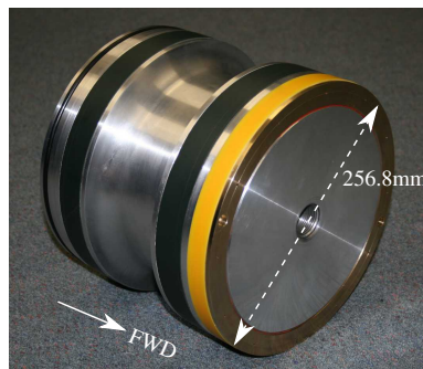
(b) Final piston assembly. Note: nylon chevron seal (yellow) and wear bands (dark green), and copper alloy seal support ring.
