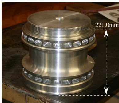
(a) Piston body, machined from 7075-T6 aluminium. Note: material removal across piston skirt, and circumferential pocketing.
