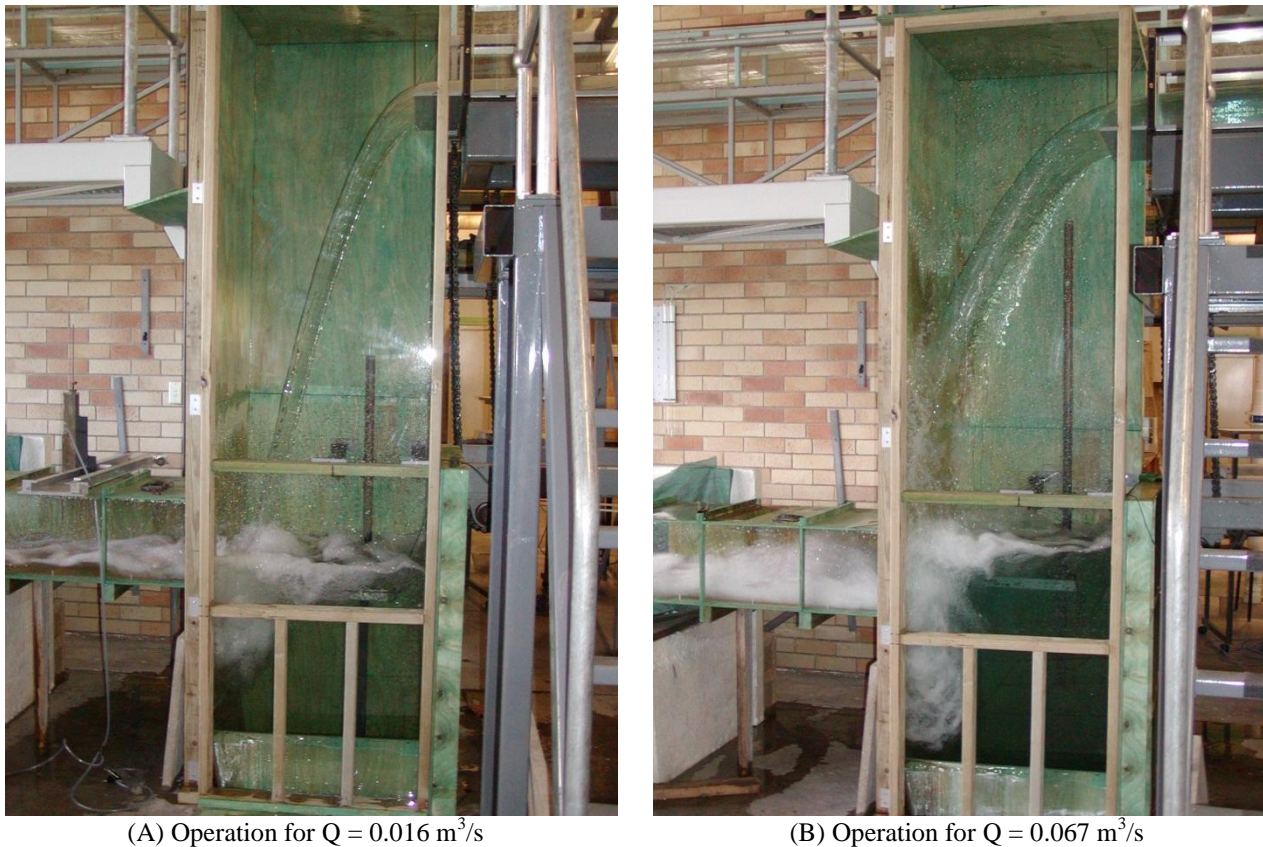
Fig. 6. Roman dropshaft in operation
