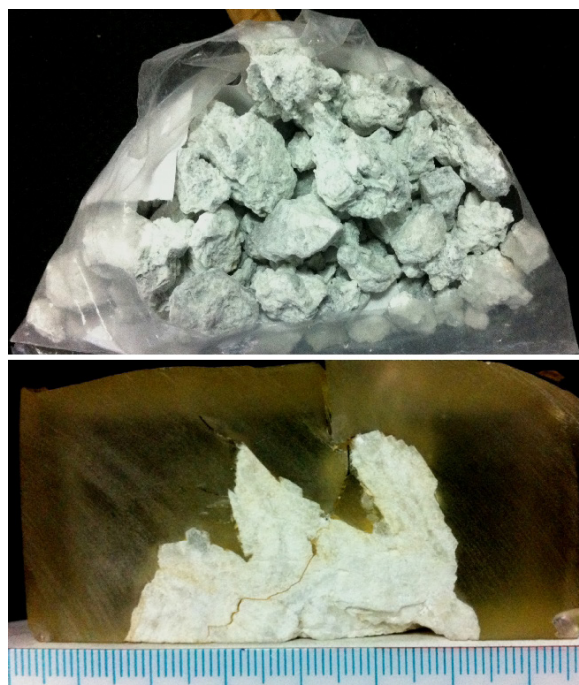
Figure 2. Images of the samples dated in this study. Up: Sample from pervasive phyllic alteration adjacent to the Villalpando vein, Sierra system; notice the green hue due to the abundance of illite. Down: Adularia sample (“valencianite”) from the La Valenciana ore shoot of the Veta Madre system.
