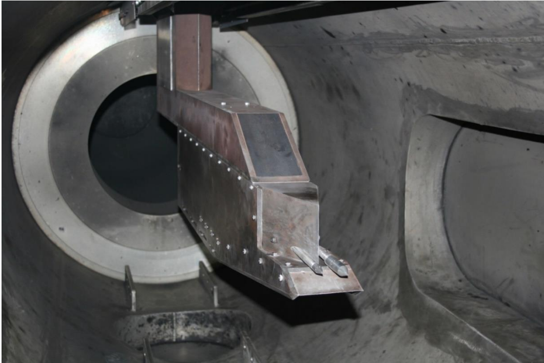
2 D scramjet in test section
