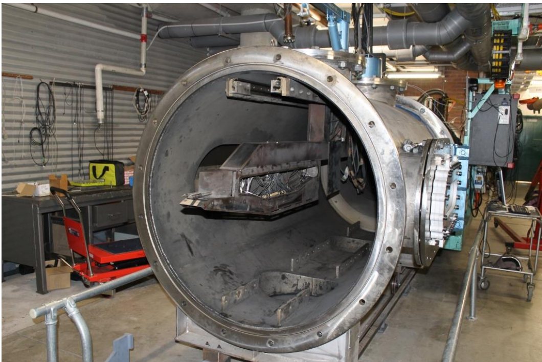
2D scramjet in test section
