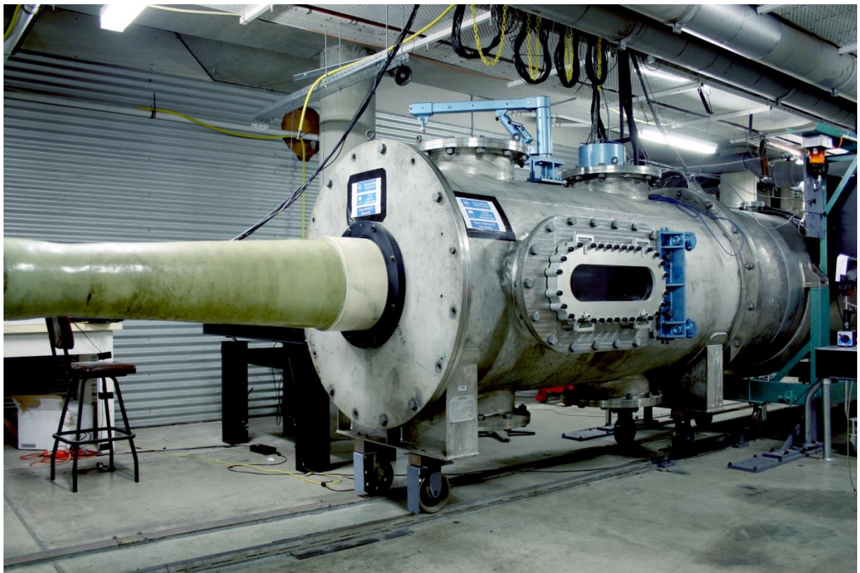
Test section with Mach 10 expansion tunnel nozzle installed.
