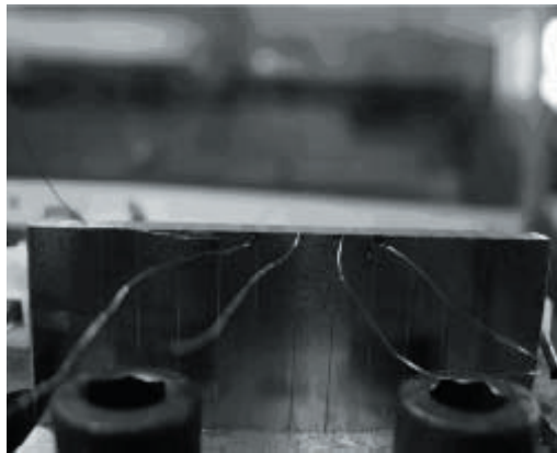
Fig. 1. Schematic drawing of the temperature measurement setup (a) and workpiece with welded thermocouples (b)
