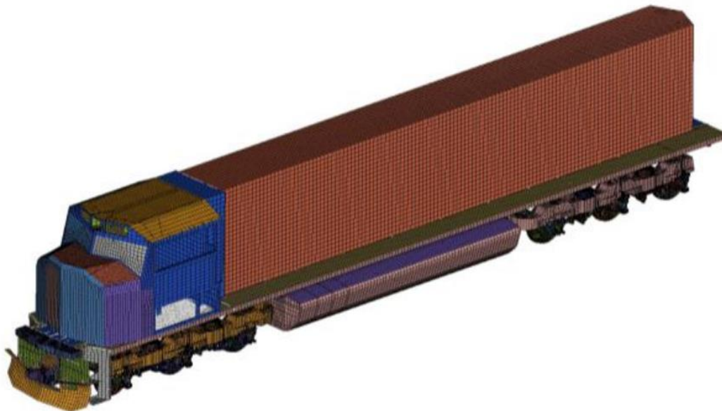
Figure 4 : FEM model of locomotive [11]
