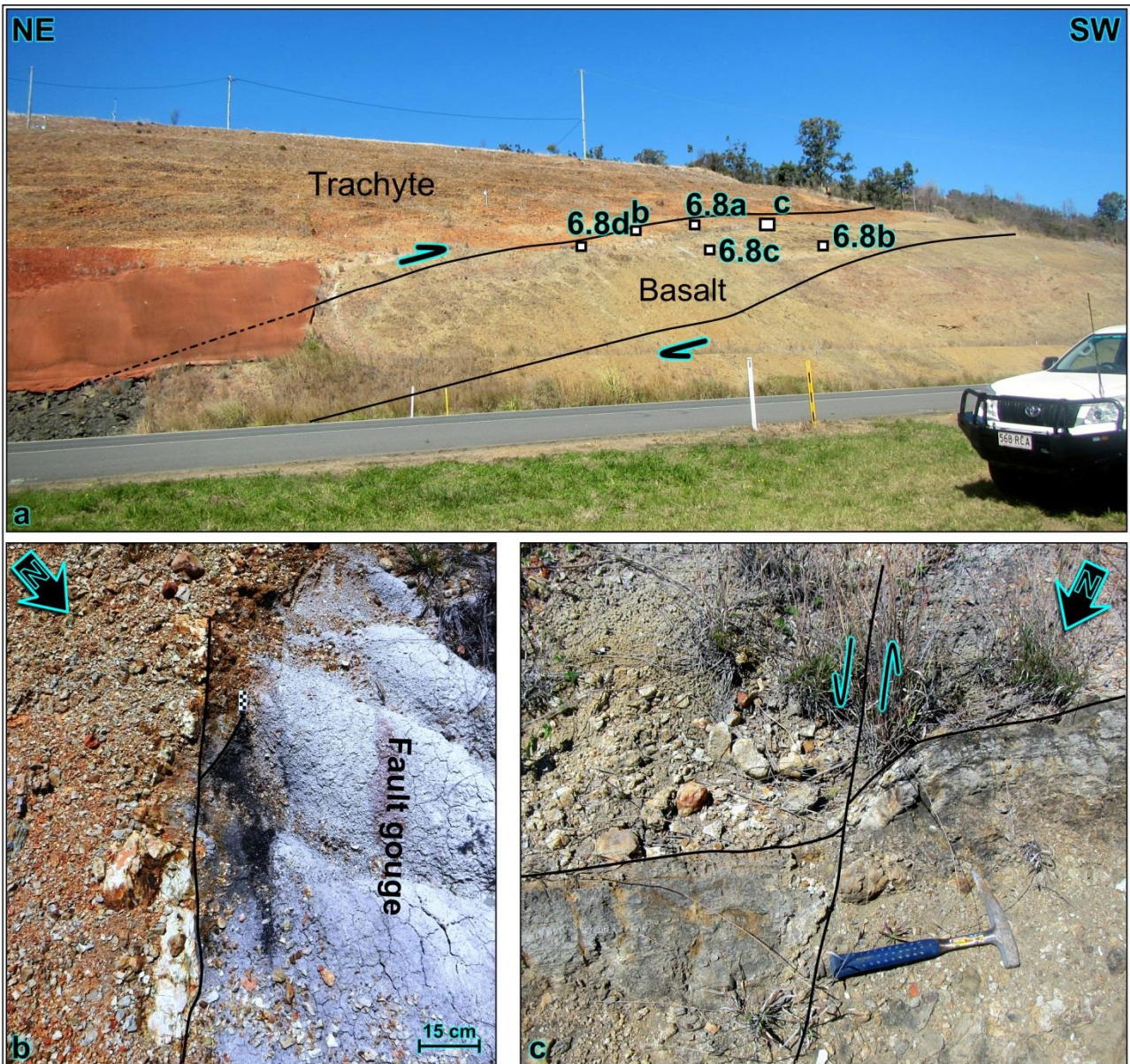
Figure 6.7. (a) The NE-striking dextral RPF, deforming Cenozoic trachyte and basalts (see Figure 6.6a for location) (X: 152°52', Y: -27°39'). (b) Fault gouge developed in the RPF zone. (c) A minor NNW-striking fault (R' shear) that displaced the main fault sinistrally.
