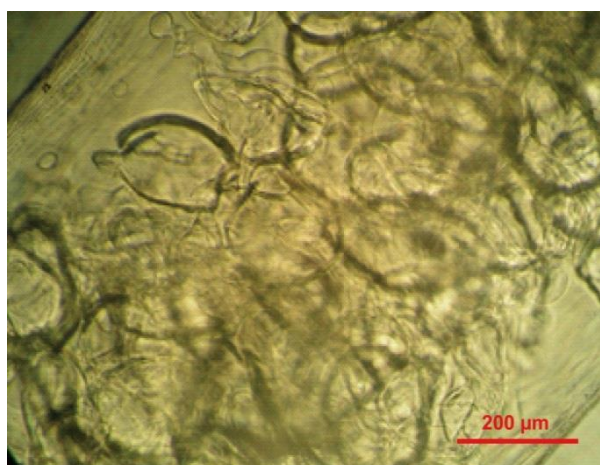
Figure 3.3 Optical micrograph of a gelatin particle-loaded alginate fibre produced by wet spinning a 57% w/w suspension of gelatin particles in alginate solution. Corresponding gelatin loading of dried spun fibre = 21% w/w.
