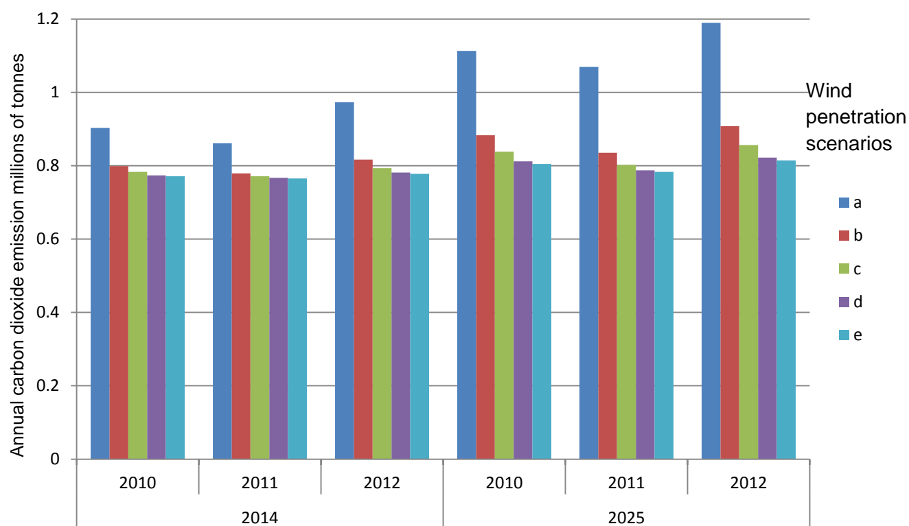
Figure 8: Comparing wind power, weather and growth effects on the TAS's annual CO 2 emissions
