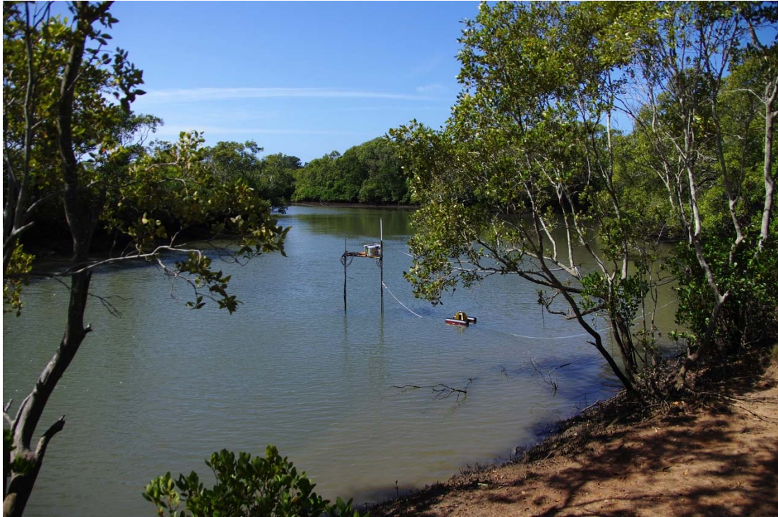
(A) Sampling site 2B view from downstream (picture from left bank) during a flood tide at about 13:47 on 29/09/2013. Note the ADV mount at the middle of the channel with YSI6600 mount moored closed to the pole.
