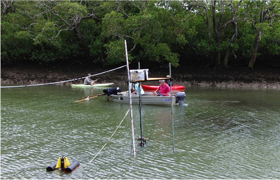
(A) Sampling location during ebb tide at 10:58 am on 30/09/2013; wind speed of about 1.3 m/s in NNE direction (i.e. blowing downstream the ADV) created energetic subsurface flow across the channel.
