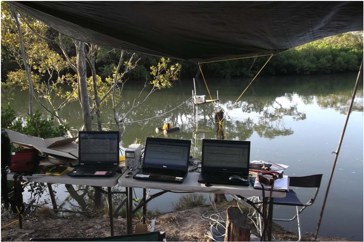
Fig. B-4 - Setup of the continuous monitoring station with a computer to an individual ADV probe. From left to right: ADV2, ADV1 and ADV3.
