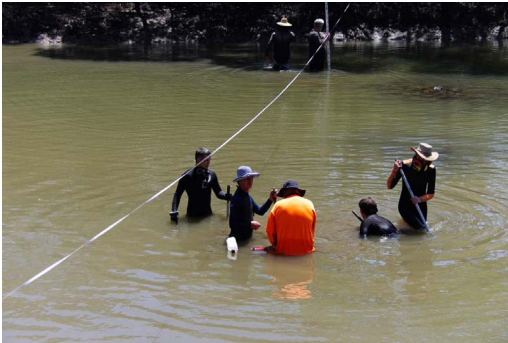
Fig. 2-7 - Research team preparing the sampling site and installing ADV mounts. In parallel, the cross-sectional survey was conducted at ADVs sampling location. View from the left bank at 12:10pm on the 29 th September 2013.
