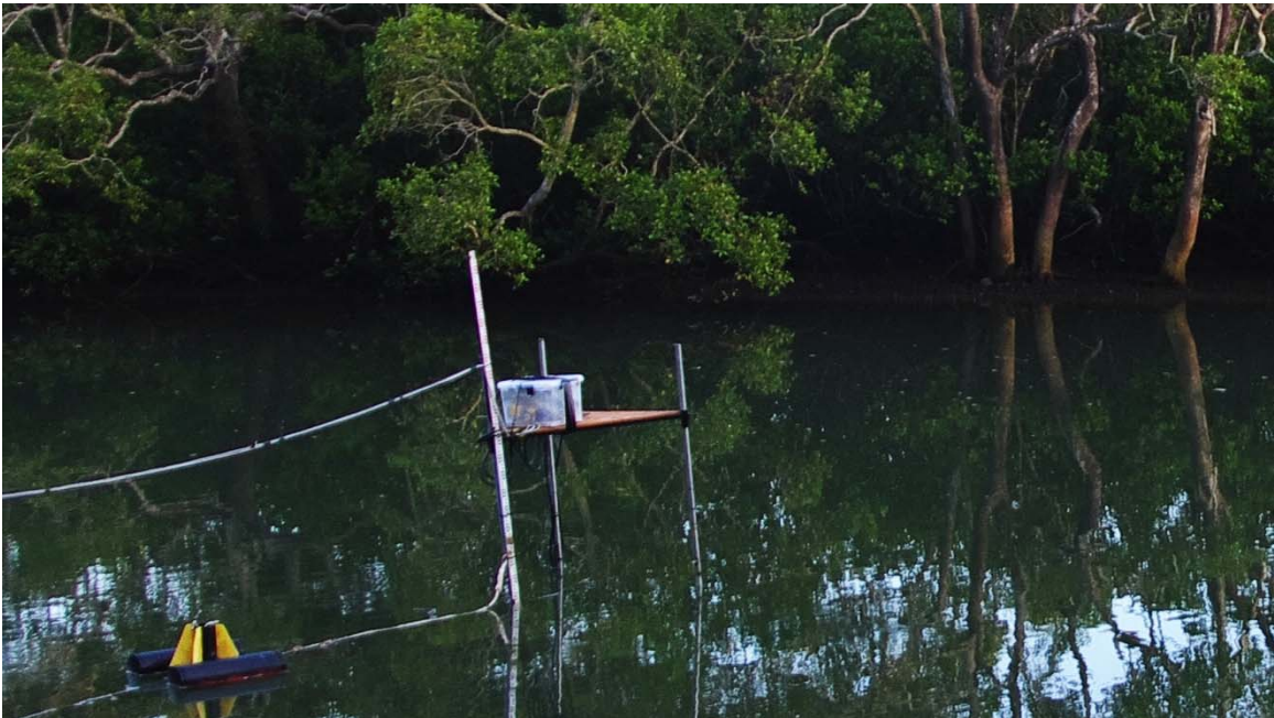
(B) Sampling location around high water slack at 5:53 am on 30/09/2013; wind was still and thus, no wind stress on subsurface layer to generate surface waves; ADVs were fully submerged: motion dominated by resonance.
