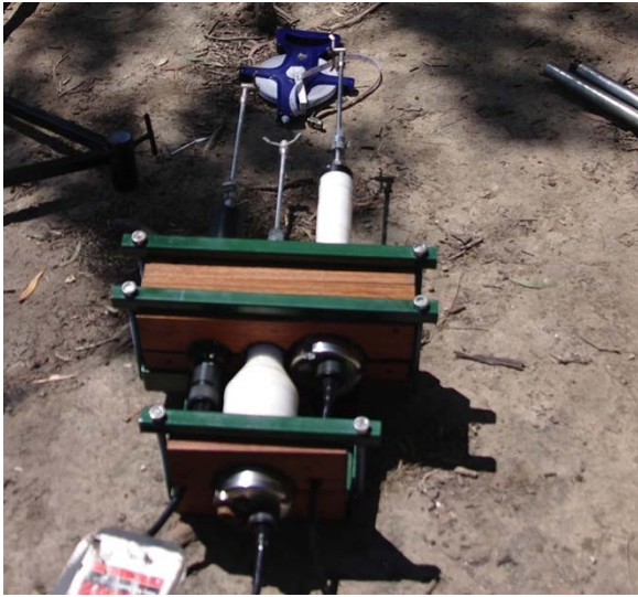
(A) Sontek® microADV 16 MHz probes
