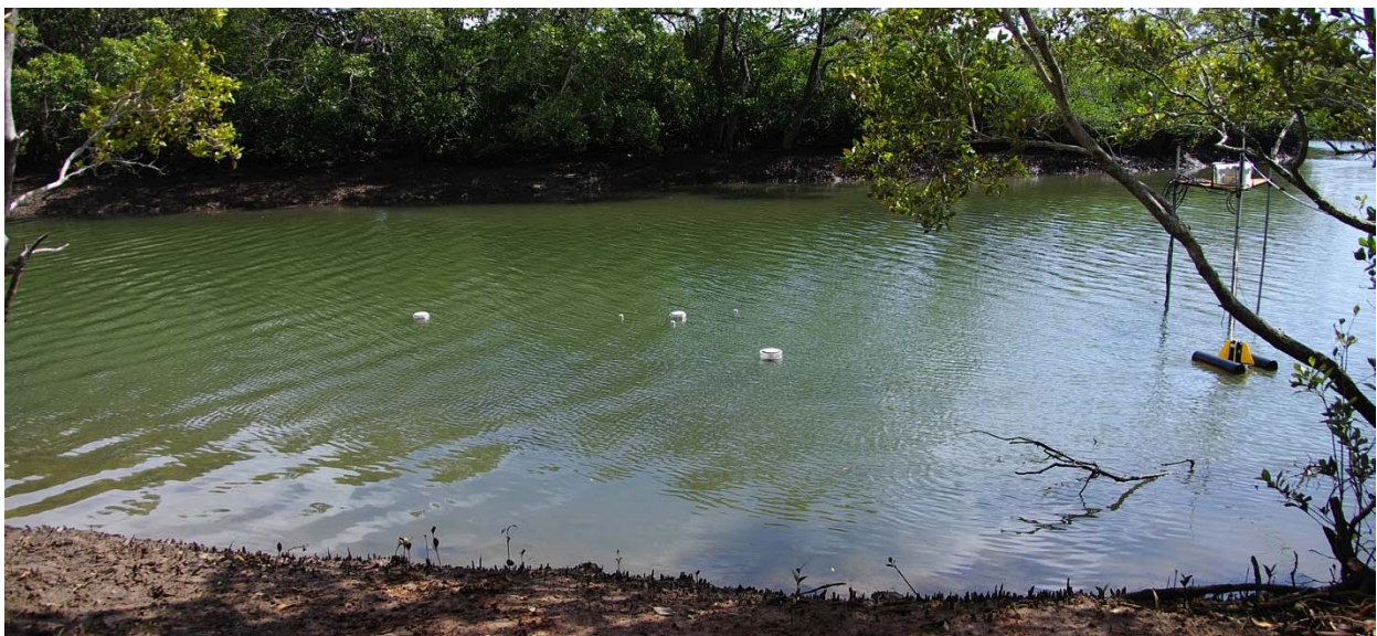
Sampling site at Erapah Creek (QLD, Australia) on 30 September 2013 at mid-ebb tide, looking from the left bank – Note the tripod holding the ADV units and the surface probe to the left, and GPS-tracked drifters at centre of the channel
