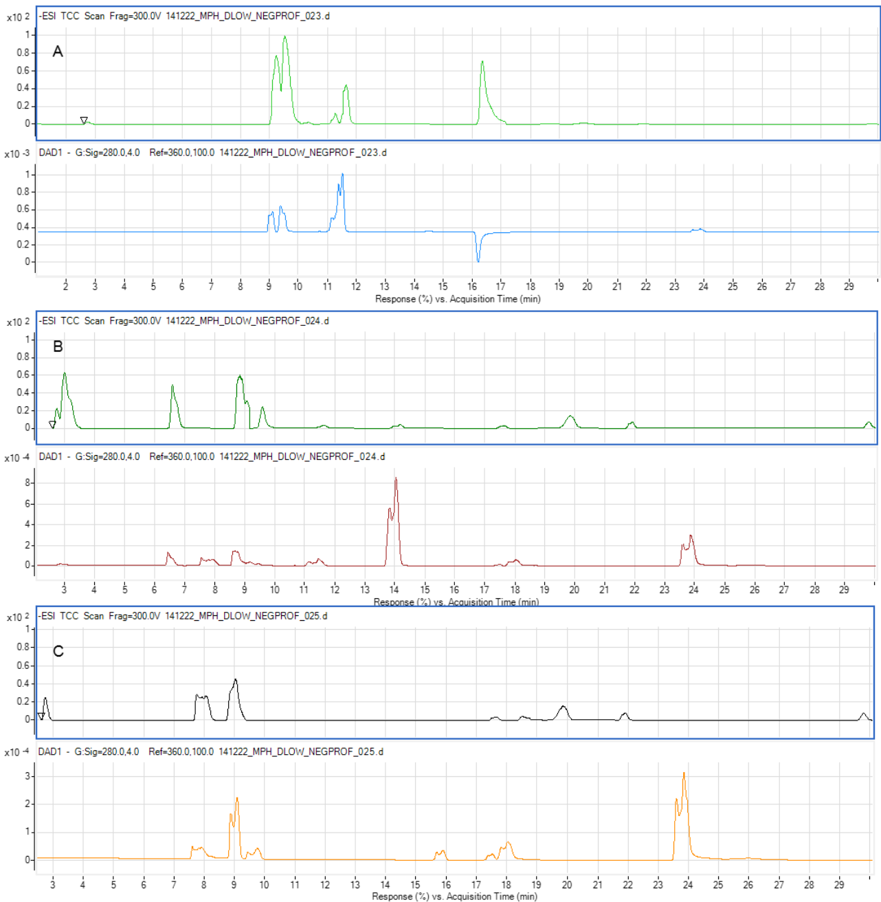
Figure A3.3. TCC and UV chromatograms of polyphenol authentic standards at 280 nm. (A) Standard mix of chlorogenic acid, coumaric acid, mangiferin, epicatechin, ferulic acid, quercetin and caffeic acid, (B) standard mix of benzoic acid, pyrogallol, 3- and 4-hydroxybenzoic acid, cinnamic acid, 4-hydroxyphenylacetic acid, protocatechuic acid, neochlorogenic acid, (C) standard mix of hippuric acid, quinic acid, syringic acid, ethyl ferulate, kaempferol, 3-(4-hydroxyphenyl)propanoic acid, 3-(3,4-dihydroxyphenyl)propanoic acid. Note that while some phenolics appear in both TCC and UV chromatograms, some compounds do not show up on the TCC or if they do, appear in extremely low intensities unless an 'Extracted Ion Chromatogram' feature was performed for a targeted m/z.
