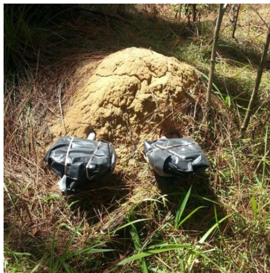
Figure 4. Photographic image of mound of termites from genus Coptotermes . The image also shows assembled devices of bait applications for termite field trial.
