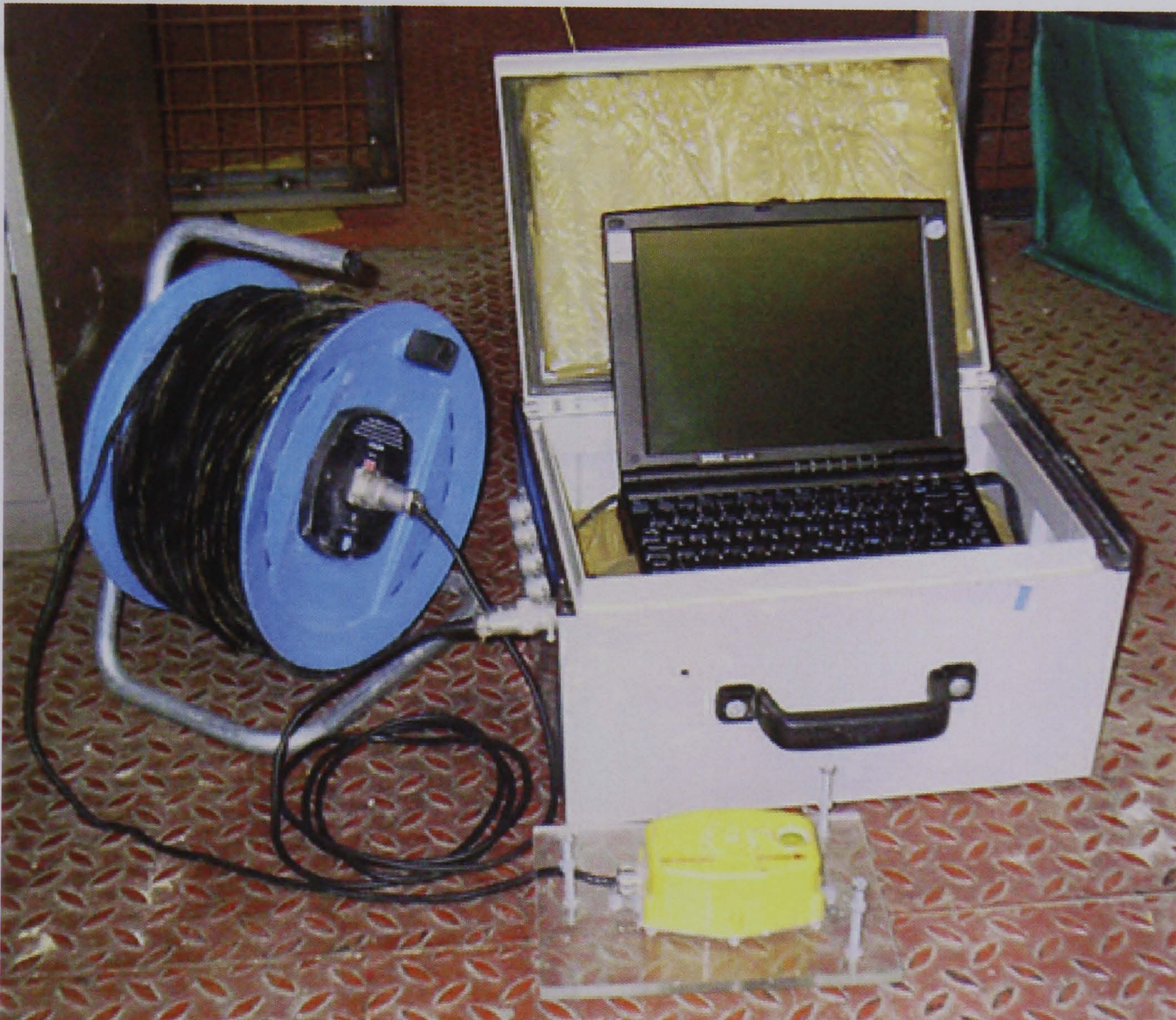
Figure 2.1 Digital Blasting Seismograph based on a laptop computer with ADC card.
