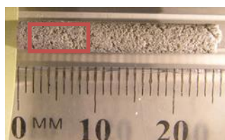
Fig. 7-8 Core photography of an Evergreen Formation sub-plug selected for high resolution micro-CT imaging (marked in red, 4.164 mm \times 4.164 mm \times 7.26 mm) (Golab, 2012; Farquhar et al., 2013; Gao et al., 2014b).
