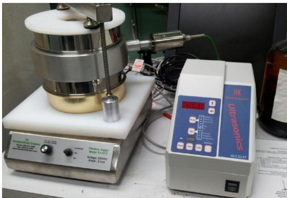
Figure 20: Sieve shaker and ultrasonic ring (left) with ultrasonic wave generator (right).
