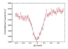
Figure 6.5: Example of observed two-photon interference between output waveguides 2 and 6 as a function of relative path difference between photon pairs input into neighbouring waveguides 1 and 2. The visibility of the dip is  $\mathcal{V}_{2,6} = 38 \pm 2\%$ , calculated from a Gaussian fit (blue line).
