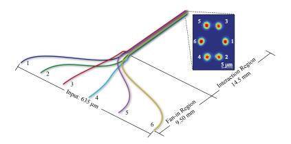
Figure 6.1: Schematic of the integrated waveguide circuit (drawing not-to-scale) and associated output. At the input the waveguides are equally spaced by 127  $\mu$  m. They then converge via a two-stage fan-in to their eventual elliptical configuration. The inset is a CCD image of the output: the waveguides are arranged with equal angular spacing around an ellipse with semi-major and semi-minor radii of 10.2 and 7.0  $\mu$ m respectively.
