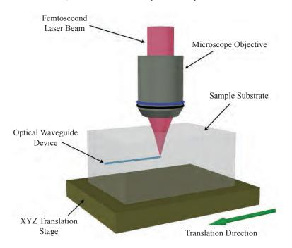
Figure 5.1: An illustration of a typical process for creating femtosecond laser-written waveguide arrays. The pulsed laser beam is tightly focused with a microscope objective into the sample, which can then be precisely translated in three dimensions to produce waveguides. This figure is reproduced from Ref. [15].
