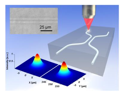
Figure 5.2: An illustrative schematic of a 50/50 laser-written directional coupler reproduced from Ref. [24]. The upper-left inset shows a microscope image of the two parallel waveguides in the interaction region, while the bottom inset shows the output mode intensity profiles.
