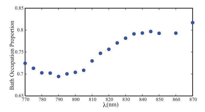
Figure 7.8: The occupancy of the bath as a function of wavelength  $\lambda$  for narrow-band (few nm) illumination for the most promising second-generation 15 cm ENAQT circuit. Note the clear minimum when  $\lambda$  is approximately 790 nm. These results suggest that this circuit may allow better ENAQT simulation with a central wavelength of  $\lambda_0=790$  nm as opposed to the design wavelength of  $\lambda_0 = 820$  nm.
