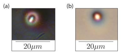
Figure 5.3: (a) Transmission differential interference microscope image of a laser written waveguide which is single mode at 800 nm prior to annealing. (b) Bright field microscope image of a different but similarly-written waveguide after annealing over a 40 hour duration. The latter is single mode at 800 nm after annealing but not before. Figure used with permission from T. Meany [36].
