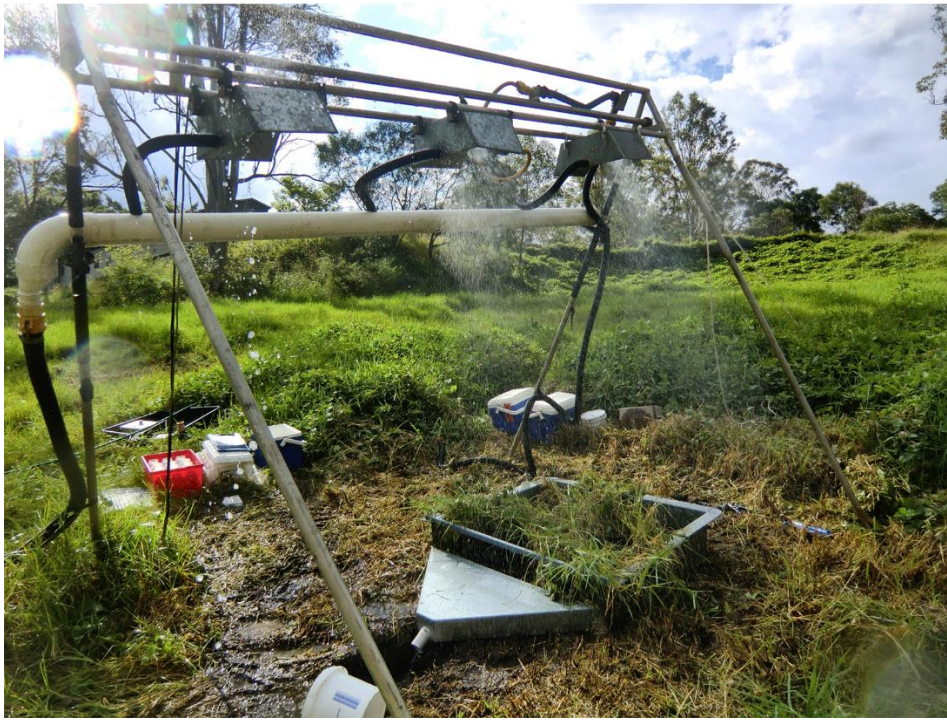
Figure 3.2 Photo of the field rainfall simulator.
