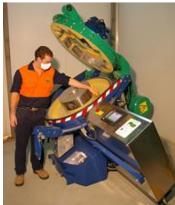
Figure 35: JK Rotary Breakage Tester (JKTech 2011)
