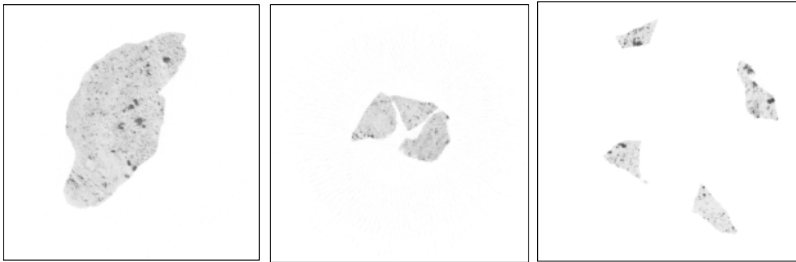
Figure 63: Sample A, parent particle (13mm); progeny particles float and progeny particles sink (-2.8mm + 2.4mm)
