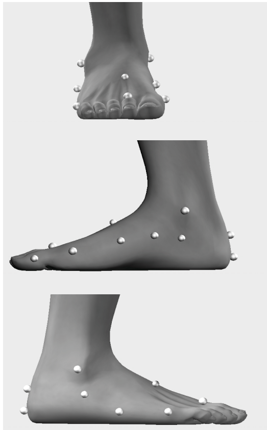
Figure 4.3. Retroreflective skin marker locations. Retro-reflective skin markers were applied to the right foot of each subject in order to create a multi-segment foot model. Views from the anterior (top), medial (middle) and lateral (bottom) aspects of the right foot. Markers are attached to rigid plastic disks and are secured to the skin with double-sided adhesive tape.
