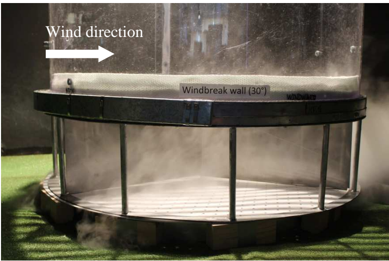
Figure 6.37. Smoke visualization in the tower base for windbreak wall angle of 30^\circ at wind speed of 2 m/s
