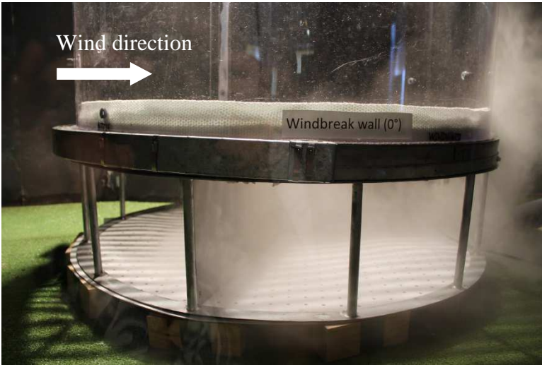
Figure 6.36. Smoke visualization in the tower base for windbreak wall angle of 0^\circ at wind speed of 2 m/s
