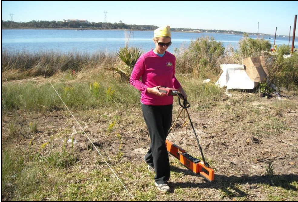
Figure 2. Geonics EM38B dual electromagnetic conductivity and magnetic susceptibility meter with data logger. Transmitter is located in the front of the instrument, receiver in back, spacing between is 1 m.
