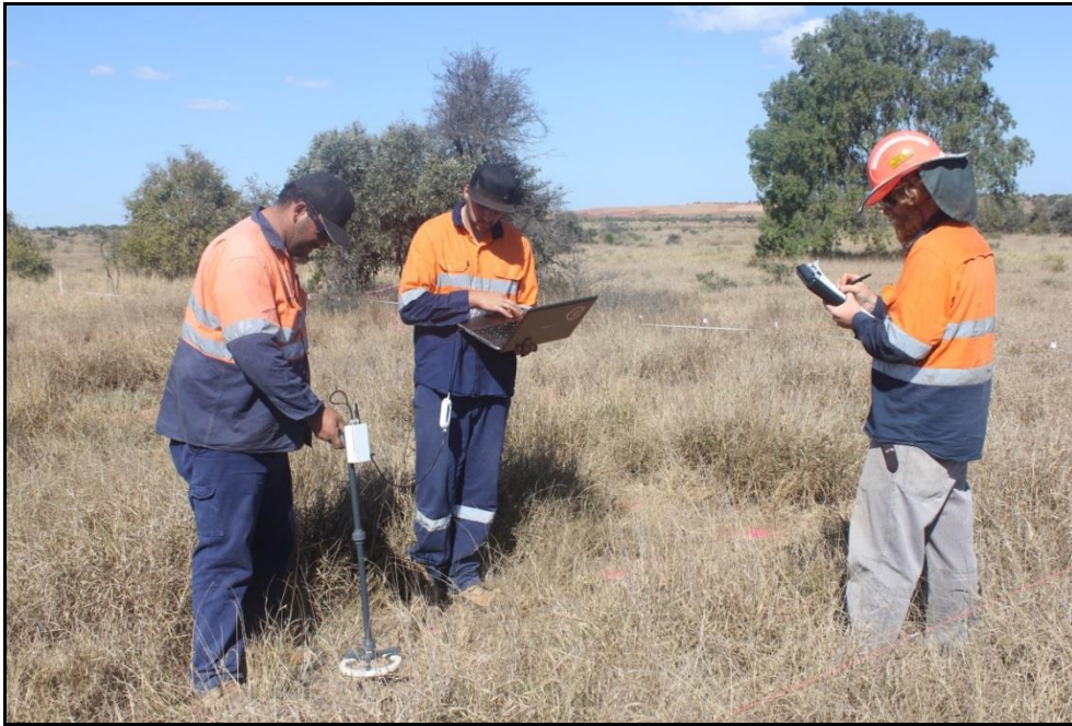
Figure 4. Bartington Instruments MS3 magnetic susceptibility meter with a MS2D field search loop (pictured left) (courtesy of Dan Rosendahl).
