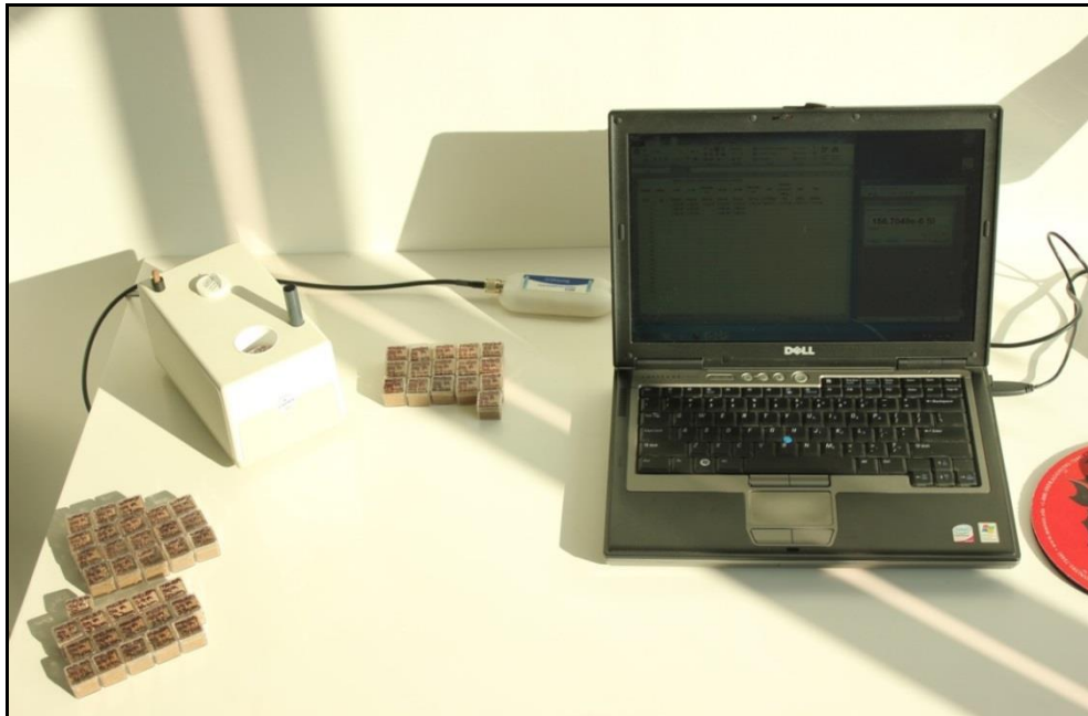
Figure 5. Bartington Instruments MS3 (top center) with MS2B lab sensor (left) and laptop computer (right). Note sediment samples packed in non-magnetic Althor P-15 boxes.
