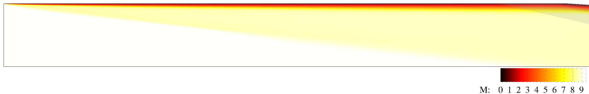
Figure 4.1: Mach number contours showing boundary layer growth along the forebody upstream of the inlet
