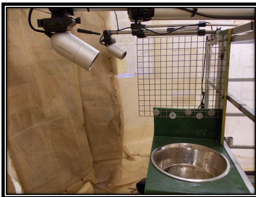
Photo 12. Mesh attached to external feed device.
