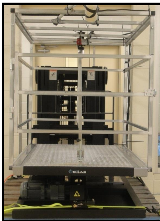
Photo 2. Crated attached to the programmable platform.
