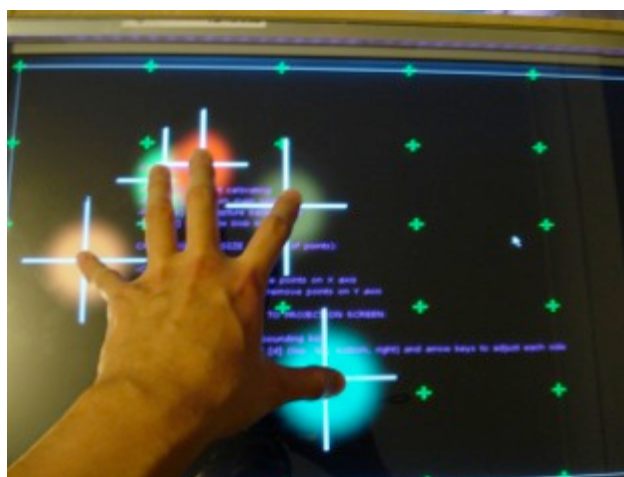
Figure 46: CCV multi-touch calibration software.
