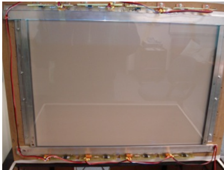
Figure 43: First attempt of the FTIR setup: embedding IR LEDs to light up the acrylic
