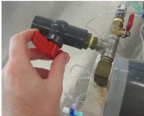
Figure 3.3: Ball valves used to lower (large valve) and raise (small valve) circulatory volume in the MCL
